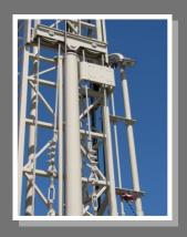
PULLDOWN/HOLDBACK: The pulldown holdback system powers the tophead rotary in either the pulldown mode or the holdback mode through the use of heavy-duty cables and a 6-1/2" (165 mm) hydraulic cylinder. Pulldown mode provides 25,000 lb. (11,340 kg) with a feed rate up to 94 FPM (28.6 MPM). Holdback mode provides 50,000 lb. (22,680kg) with a pull out rate up to 106 FPM (30.4 MPM).
