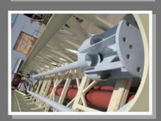
**CAROUSEL:** Heavy-duty carousel (6.08 m) drill pipe mounted in derrick. It storage in right rear corner of mast and manually controlled from working platform.
